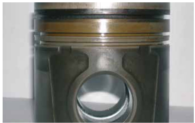
Piston with ring grooves – MWM TCG 2016 V12
